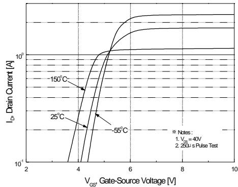
**Figure 2. Transfer Characteristics**
