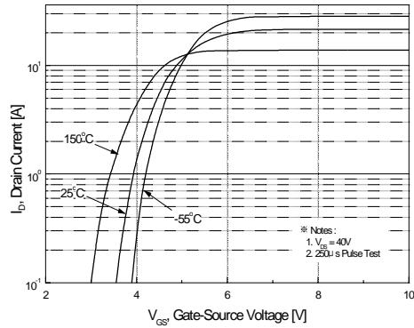
**Figure 2. Transfer Characteristics**
