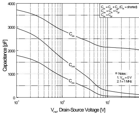
**Figure 5. Capacitance Characteristics**
