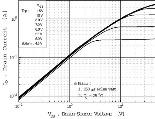
Fig 2. Transfer Characteristics
