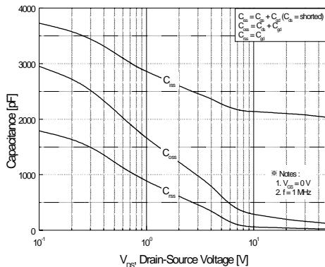
**Figure 5. Capacitance Characteristics**
