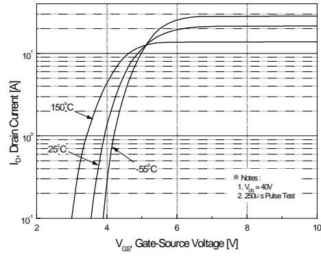
**Figure 2. Transfer Characteristics**
