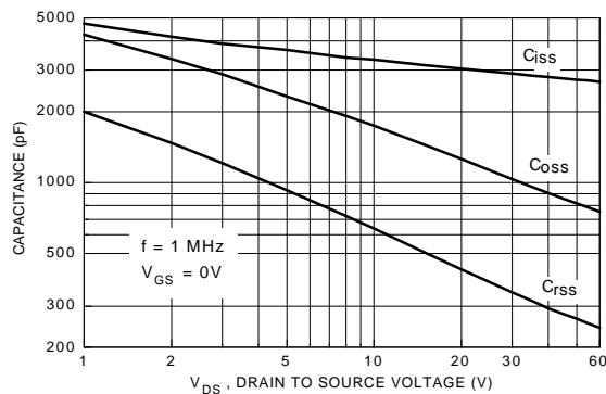
**Figure 9. Capacitance Characteristics**
