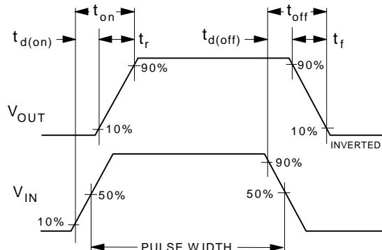
**Figure 12. Switching Waveforms**
