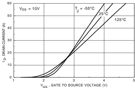
**Figure 5. Transfer Characteristics.**
