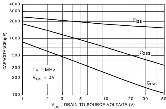
**Figure 9. Capacitance Characteristics.**
