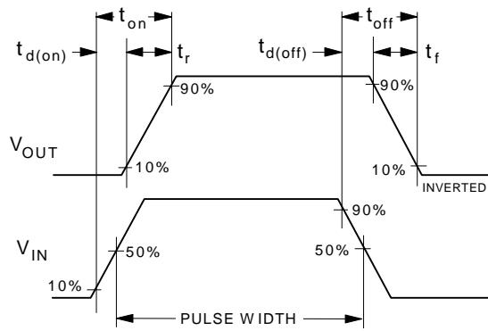
**Figure 12. Switching Waveforms.**
