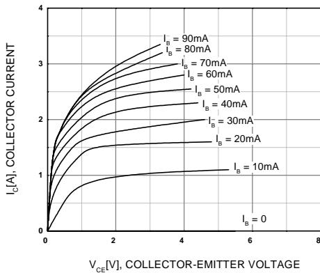
Figure 1. Static Characteristic
