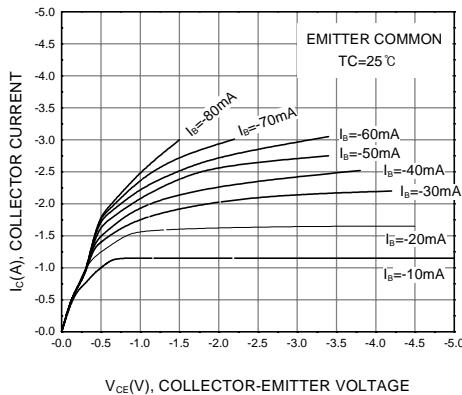
Figure 1. Static Characteristic
