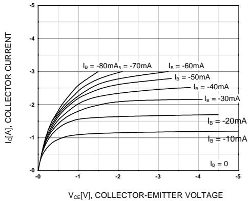
**Figure 1. Static Characteristic**
