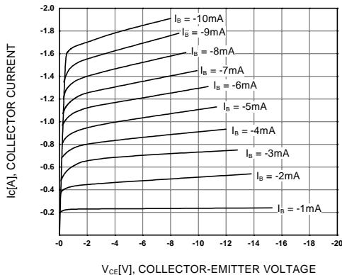
**Figure 1. Static Characteristic**
