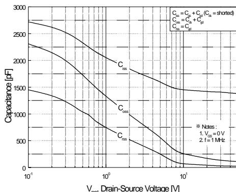
**Figure 5. Capacitance Characteristics**
