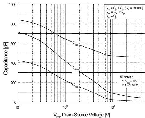
**Figure 5. Capacitance Characteristics**
