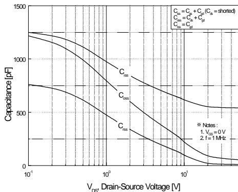
**Figure 5. Capacitance Characteristics**
