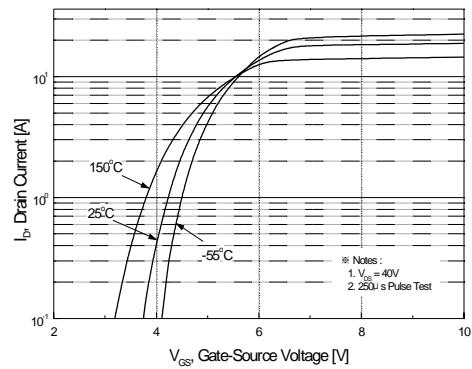
**Figure 2. Transfer Characteristics**
