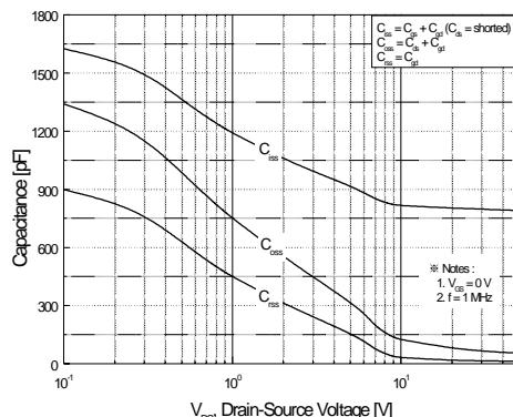
**Figure 5. Capacitance Characteristics**
