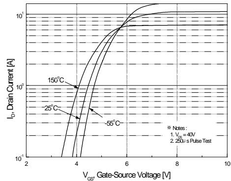
**Figure 2. Transfer Characteristics**
