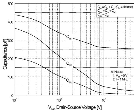
**Figure 5. Capacitance Characteristics**
