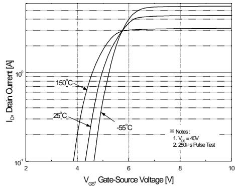
**Figure 2. Transfer Characteristics**
