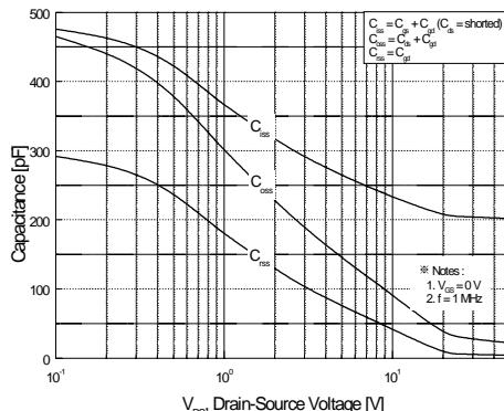
**Figure 5. Capacitance Characteristics**
