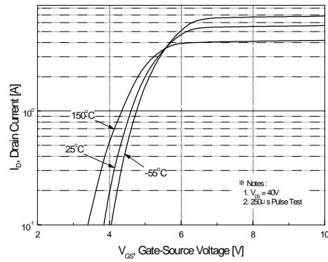
**Figure 2. Transfer Characteristics**
