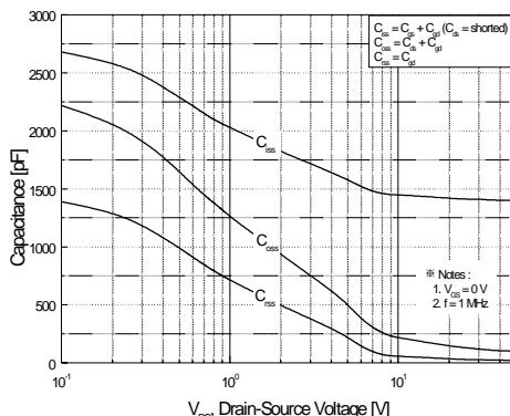
**Figure 5. Capacitance Characteristics**
