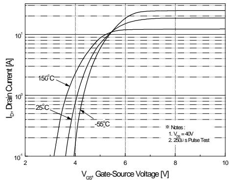
**Figure 2. Transfer Characteristics**
