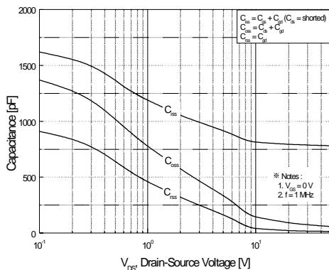
**Figure 5. Capacitance Characteristics**
