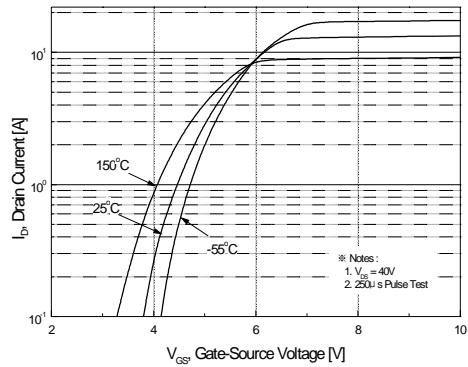
**Figure 2. Transfer Characteristics**
