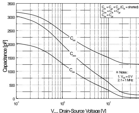
**Figure 5. Capacitance Characteristics**
