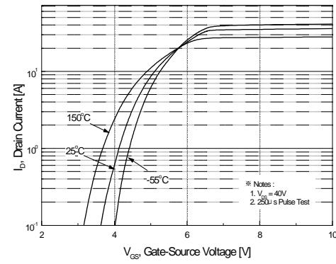
**Figure 2. Transfer Characteristics**
