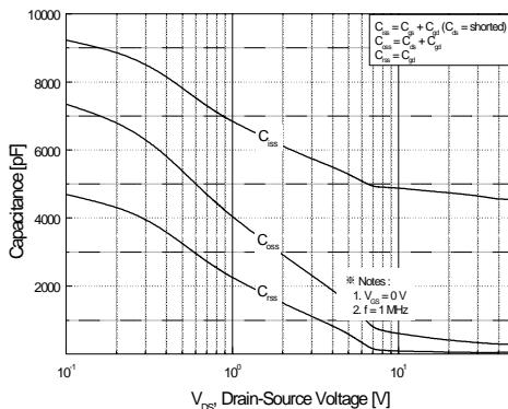
**Figure 5. Capacitance Characteristics**
