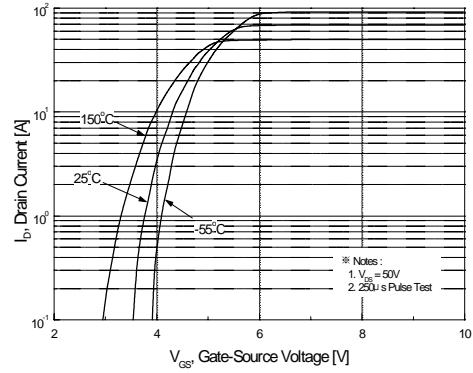
**Figure 2. Transfer Characteristics**
