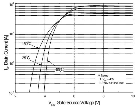
**Figure 2. Transfer Characteristics**
