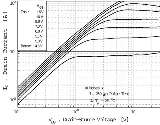
Fig 2. Transfer Characteristics
