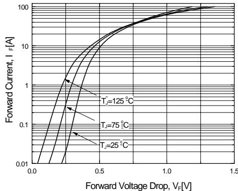
**Figure 1. Typical Forward Voltage Characteristics (per diode)**
