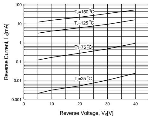
**Figure 2. Typical Reverse Current
