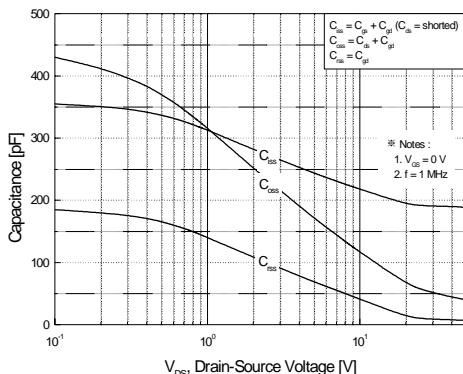
**Figure 5. Capacitance Characteristics**
