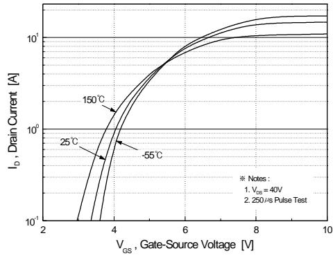
**Figure 2. Transfer Characteristics**
