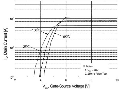
**Figure 2. Transfer Characteristics**
