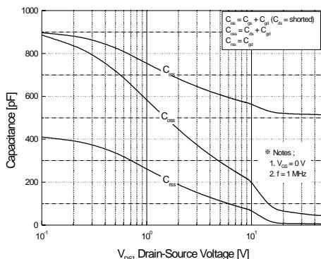
**Figure 5. Capacitance Characteristics**
