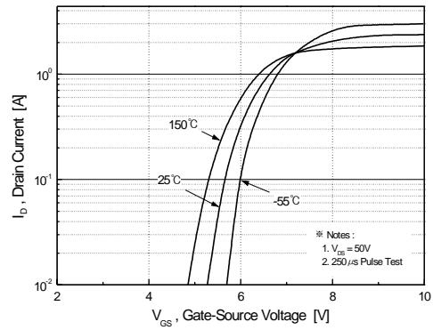
**Figure 2. Transfer Characteristics.**
