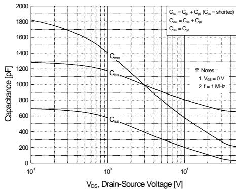
**Figure 5. Capacitance Characteristics**
