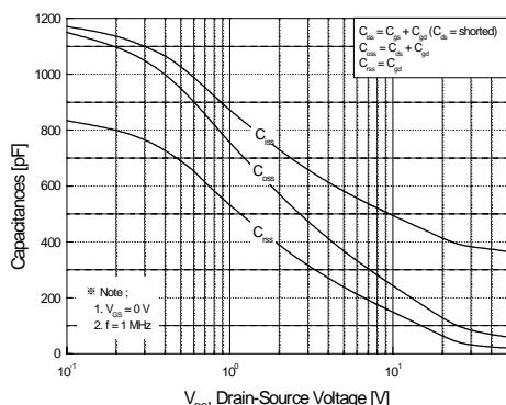
**Figure 5. Capacitance Characteristics**
