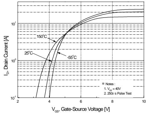
**Figure 2. Transfer Characteristics**
