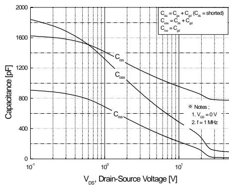
**Figure 5. Capacitance Characteristics**
