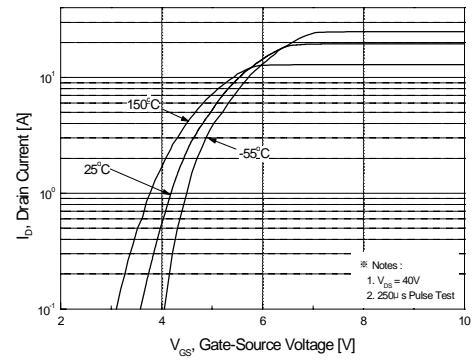
**Figure 2. Transfer Characteristics**
