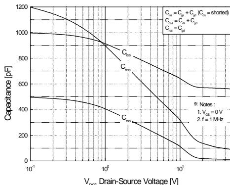
**Figure 5. Capacitance Characteristics**
