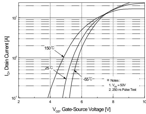
**Figure 2. Transfer Characteristics**
