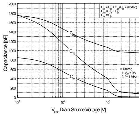
**Figure 5. Capacitance Characteristics**
