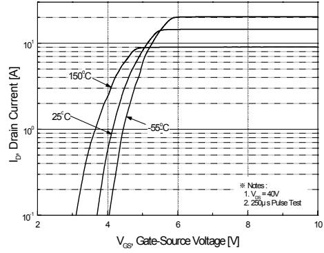
**Figure 2. Transfer Characteristics**
