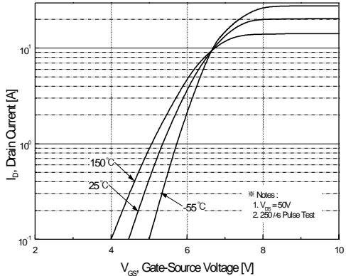
**Figure 2. Transfer Characteristics**
