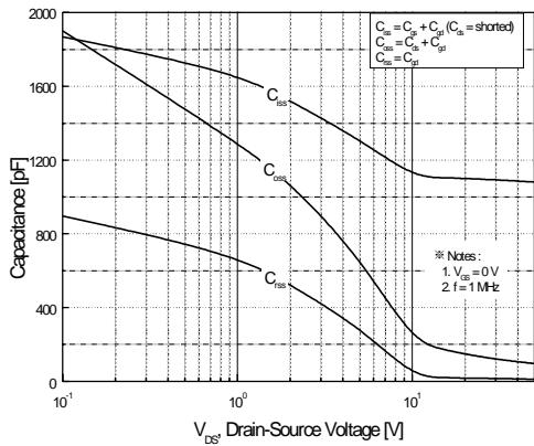
**Figure 5. Capacitance Characteristics**
