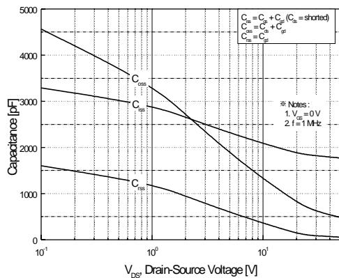
**Figure 5. Capacitance Characteristics**
