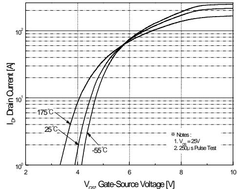
**Figure 2. Transfer Characteristics**
