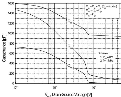
**Figure 5. Capacitance Characteristics**
