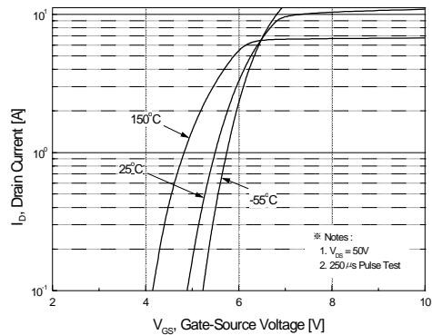
**Figure 2. Transfer Characteristics**
