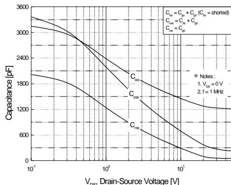
**Figure 5. Capacitance Characteristics**
