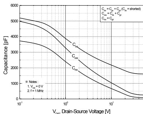
**Figure 5. Capacitance Characteristics**
