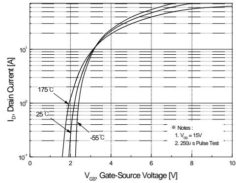
**Figure 2. Transfer Characteristics**
