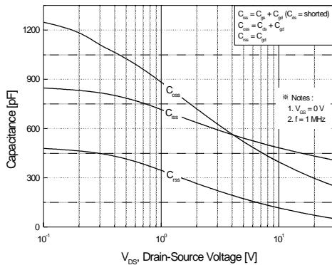
**Figure 5. Capacitance Characteristics**
