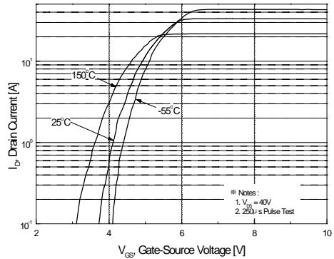
**Figure 2. Transfer Characteristics**
