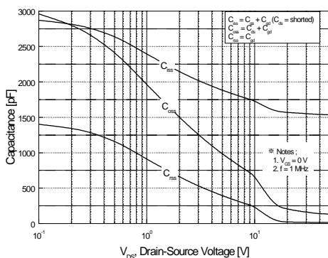
**Figure 5. Capacitance Characteristics**
