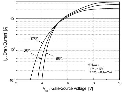
**Figure 2. Transfer Characteristics**
