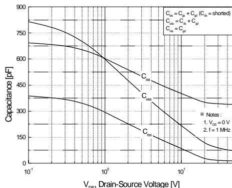
**Figure 5. Capacitance Characteristics**
