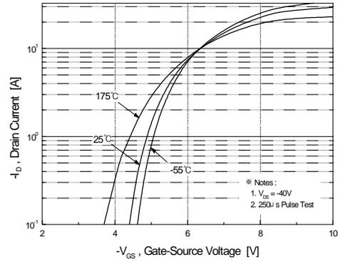
**Figure 2. Transfer Characteristics**
