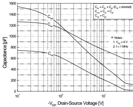
**Figure 5. Capacitance Characteristics**
