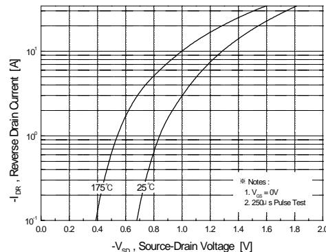
Figure 4. Body Diode Forward Voltage
