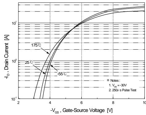
Figure 2. Transfer Characteristics
