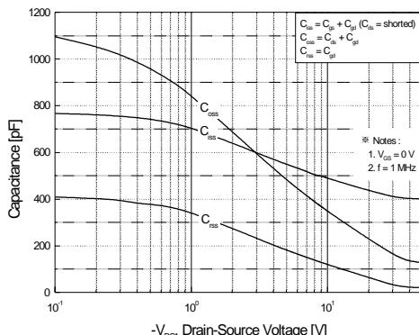
Figure 5. Capacitance Characteristics
