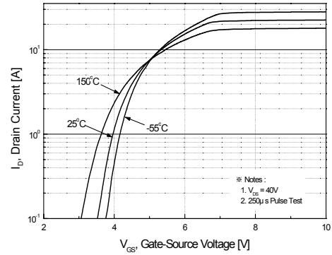
**Figure 2. Transfer Characteristics**
