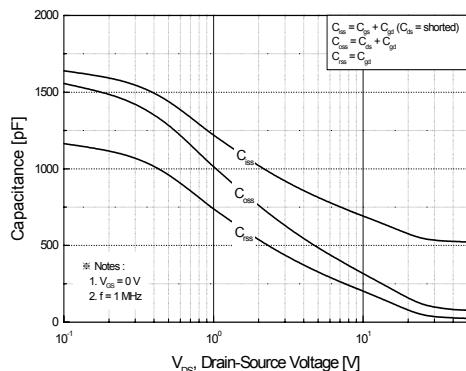
**Figure 5. Capacitance Characteristics**
