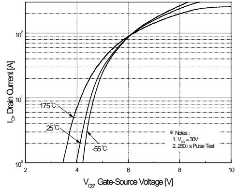
**Figure 2. Transfer Characteristics**
