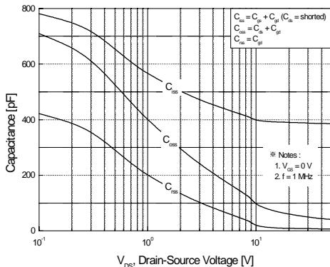
**Figure 5. Capacitance Characteristics**
