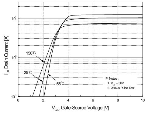
**Figure 2. Transfer Characteristics**
