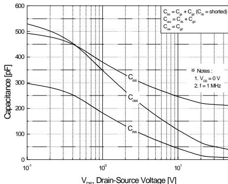
**Figure 5. Capacitance Characteristics**
