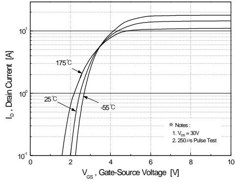
**Figure 2. Transfer Characteristics**
