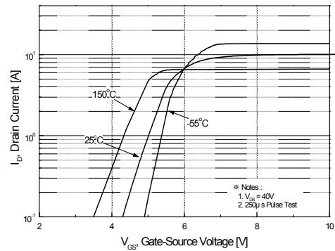
**Figure 2. Transfer Characteristics**
