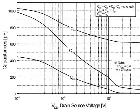
**Figure 5. Capacitance Characteristics**
