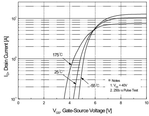
**Figure 2. Transfer Characteristics**
