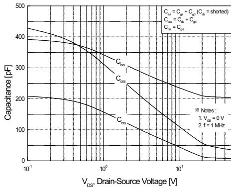
**Figure 5. Capacitance Characteristics**
