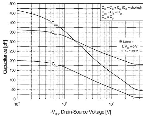
Figure 5. Capacitance Characteristics
