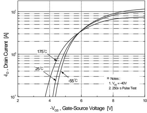
Figure 2. Transfer Characteristics
