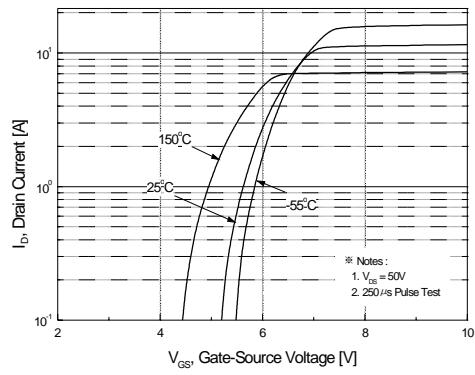
**Figure 2. Transfer Characteristics**
