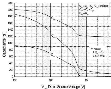
**Figure 5. Capacitance Characteristics**
